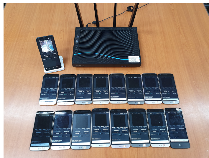
(a) Distributed system with 16 worker nodes
