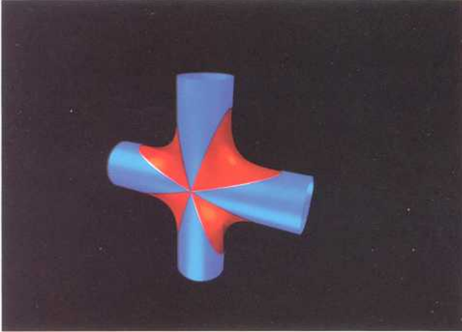
Fig. 7. Smooth blending of two cylinders with a quadric surface.
