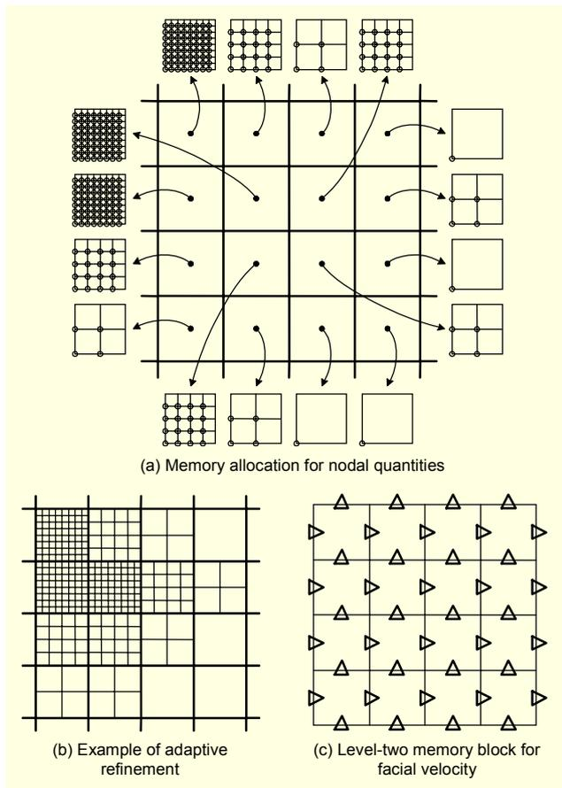
Fig. 1. Adaptive mesh representation scheme.
